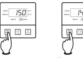
Figure 4.1 Establishing the Set Point
